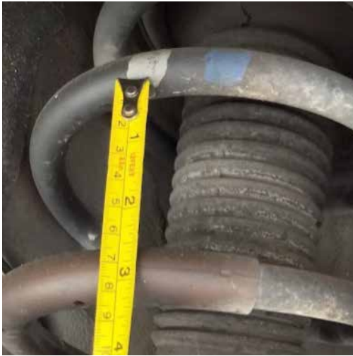
1. Jack up car, measured ~ 2.5" Gap
