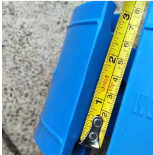
2. Choose A+ , Inner Groove is 2.5", match to Gap 2.5"
