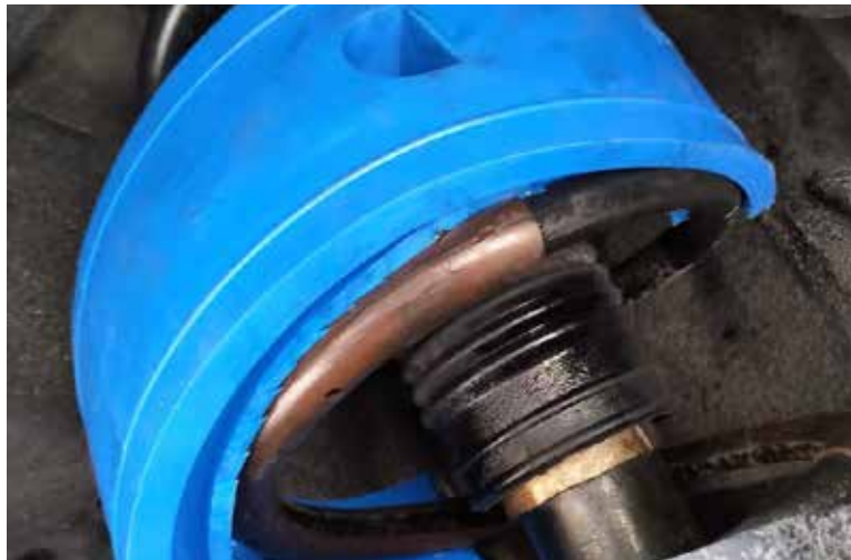
5. Choose the biggest coil gap to begin insert from top groove sit inside groove, then bottom groove pushing in. Make sure top & bottom groove bot sit on coil spring
