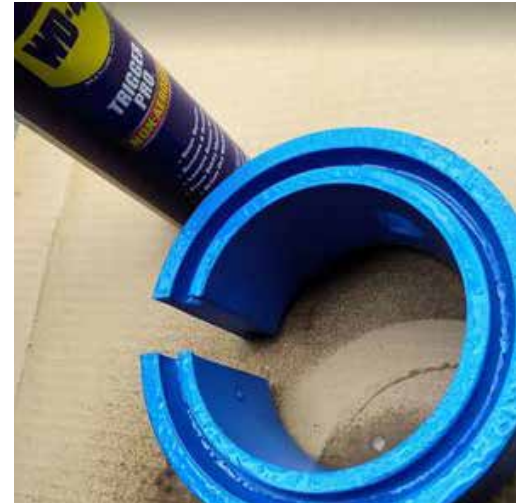
3. Spray lots of WD40 both side for easy install
