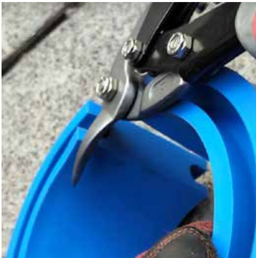
4. Cut off bottom side inner groove for easy insertion
