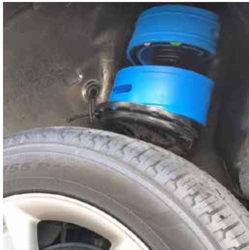
Rear coil springs : DuraTPEPlus A / BP installed
