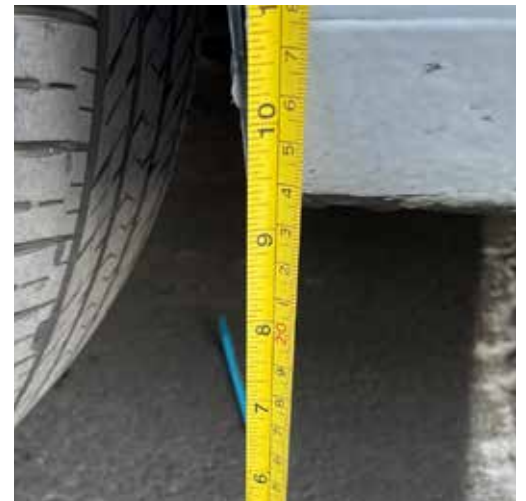
We got around 0.9" ground clearance after installation.
