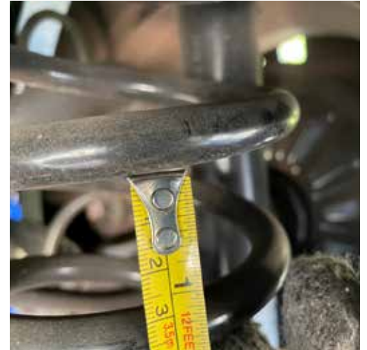
5. The rear coil springs gap is around 1.1".
