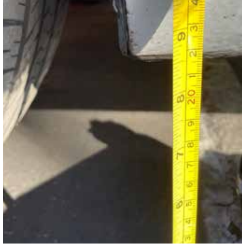
1. Before installation the ground clearance is around 10" to the reference line
