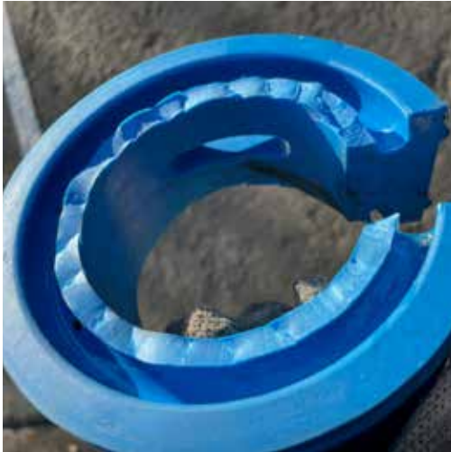
3. To ease out the installation, the top inner rings were cut off
