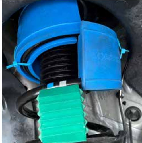
4. We install DuraTPE CSBPlus-A and Rubber Block RB275-2-175 (2" side) in the front coil springs
