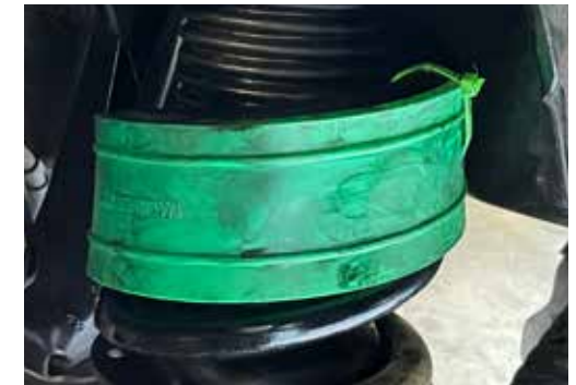
5. Front coil spring buffers installation completed, zip ties included to secure buffer in place.
