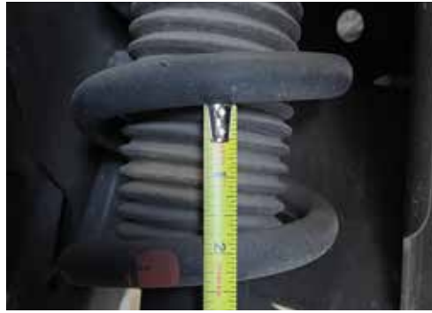
2. You will Jack up the vehicle please secure SUV using Jack Stands. The Spring will decompress and you will need to measure the gap between the springs it will give us 1.6".
