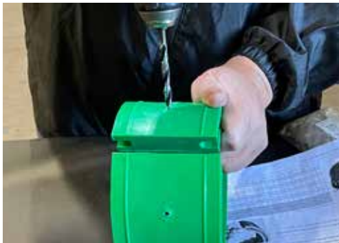
3A. CSBSuper series need to drill a 1/2" hole along the center line and 2" away from the edges
