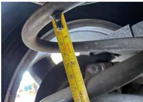
6. Measure rear coil springs gap. Gap measurement is 2.5".
