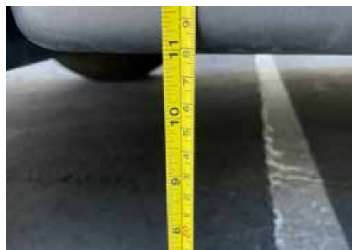
10. Ground clearances increase one inch from 10" to 11"
