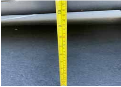
1. Vehicle ground clearance before installation is 10"
