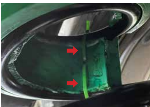
9. Because both top and bottom rings Trimmed off, we recommend to apply two extra zip ties on each hole and tie the buffer on both top and bottom coil springs after installed buffers. (only 2 zipties per buffer included.)
