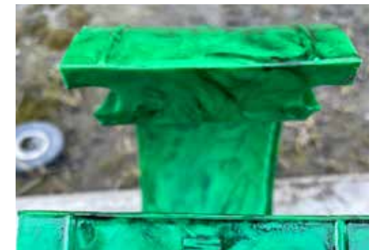
8. Due to the H2=2.36" is very close to Gap of 2.5", Both top and bottom inner rings were trim off.
