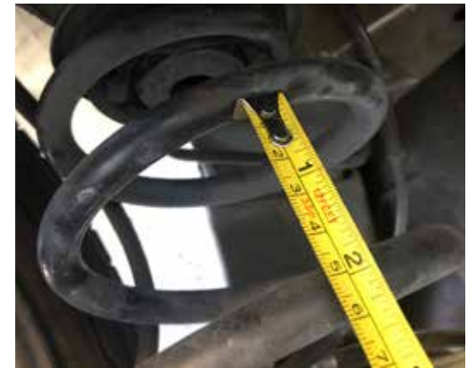
6. The rear coil spring gap D of the car is around 1.8". CSBPro-BP Size B+ of the pro series was chose
