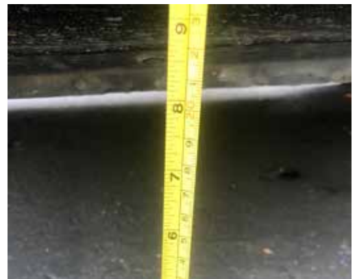
9. The vehicle ground clearance was measured 8.2" after installation. There is around 1" lift for this combination of RubberShox DuraTPE buffers and Rubber Block Boosters
