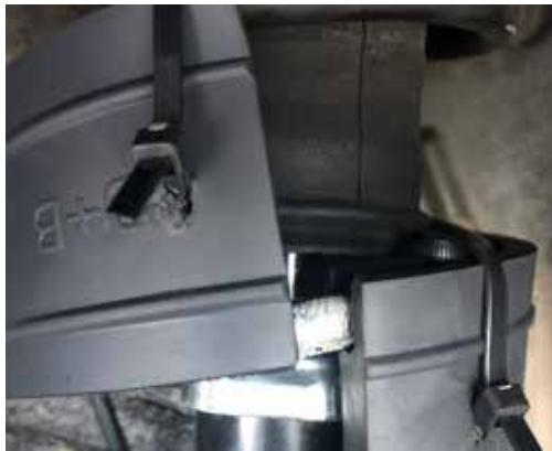
4. 1/4" diameter holes are drilled in the center line and 1-2 inches away from the open edges Buffers were tied to the top coil on both end with included zip ties
