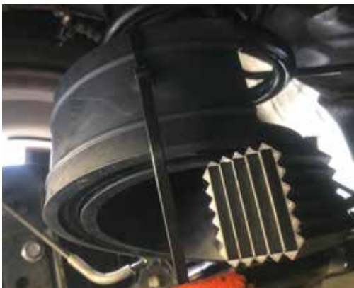
7. Buffers were tied on top of the coil and Rubber Block Booster RB2-15-125 is also installed underneath the buffers.
