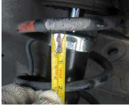
2. Measure the front coil spring gap D of the car. 1.75". Customer want firmer and more lift on the car, so CSBPro series was chosen
