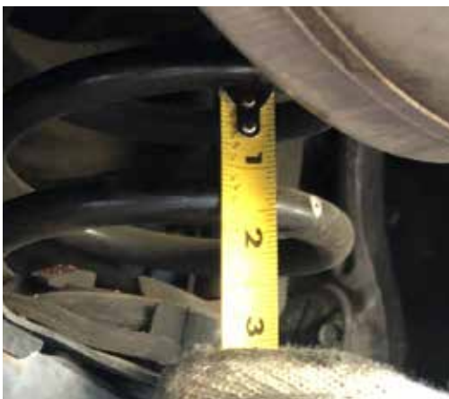
6. Rear coil spring gap is 1.1", we will use CSBPlus-C (60HA size C) for a little softer ride for back seat passengers.
