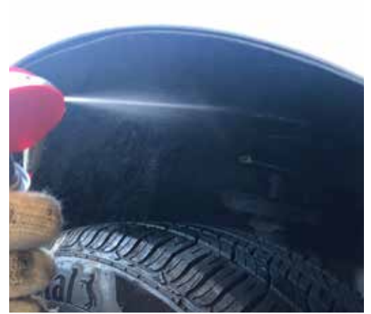
3. Use WD-40 to lube the coil springs. Please spray evenly to coil spring
