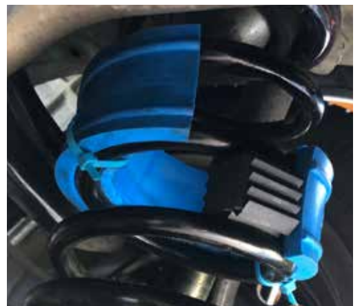
8. RB125-1-1 rubber block boosters are also added to reinforce the opening of the buffer. This block will not only make firmer control of the vehicle and add even more ground clearance
