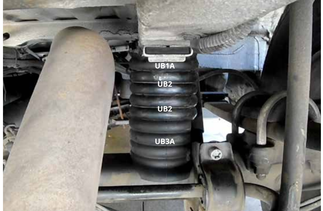
Case 1 Installed Items : Modular Universal Rubber Bump Stops UB1A223A (UB1A+UB2+UB2+UB3A) Ground Lifting Height : 2.3"
