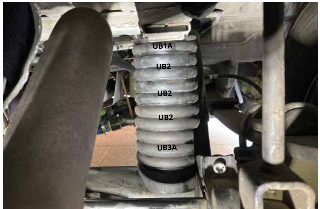
Case 2 Installed Items : Modular Universal Rubber Bump Stops UB1A2223A (UB1A+UB2+UB2+UB2+UB3A) Ground Lifting Height : 2.65"
