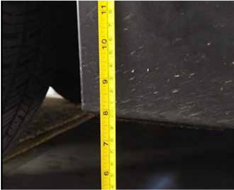
Front Suspension : Ground clearance before installation 7"
