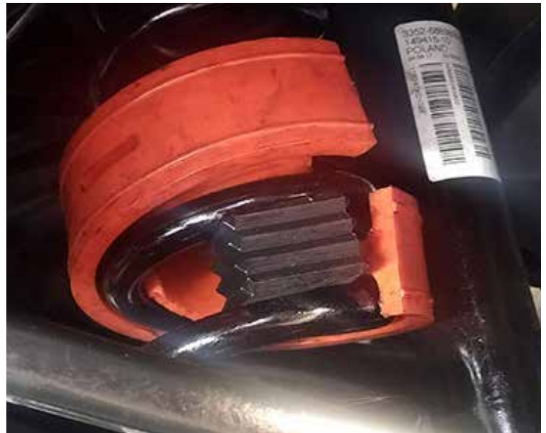
Reat Suspension : Ground clearance Lift 1.5"
