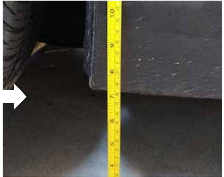
Front Suspension : Ground clearance before installation 7.9"
