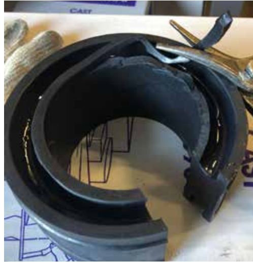
The rear installation will required cutting off the top inner ring to get a very tight fit and easier installation.
