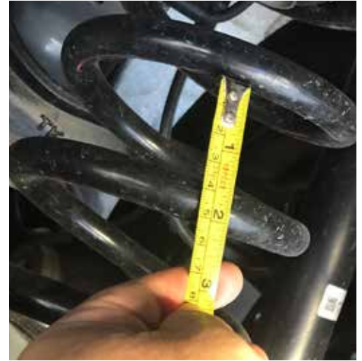
The front gap was measured 1.6" and the rear end gap is 1.35"
