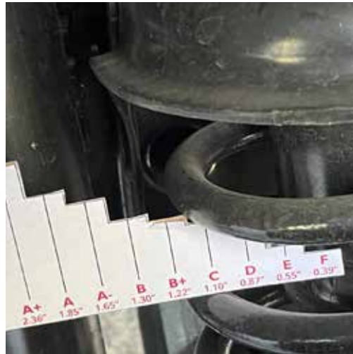
3. Using the template download from website or amazon, we choose CSBPlus-C size C for this front installation.
