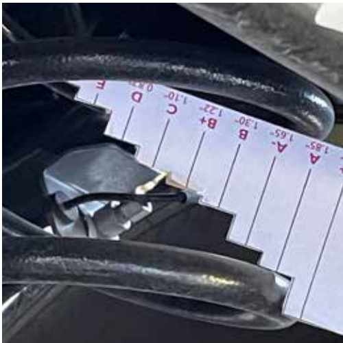
5. Using the template to decide the rear coil spring size is A
