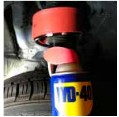
Spray WD40 on both Vehicle Coil Springs and Buffer Groove for Easier Installation
