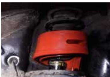
2005 Lexus RX330 Size : A+ (Front) , A (Rear) Ground Lifting Height : up to 1" (2.54cm)
