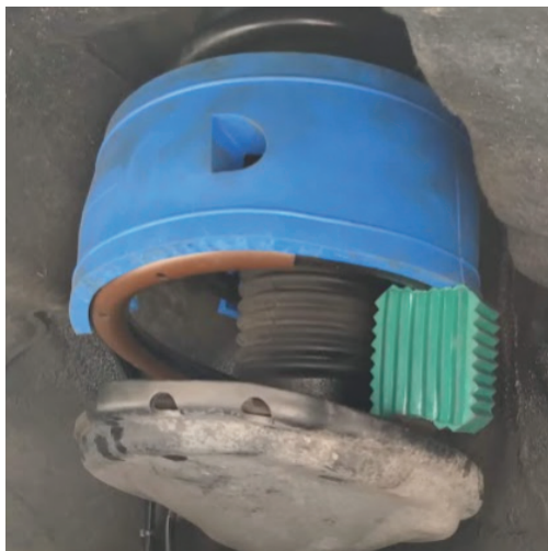
Front coil springs : DuraTPE Plus AP / Rubber Block Booster RB275-2-175 installed
