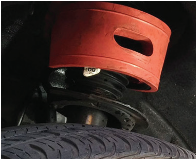
Front Suspension : Ground clearance before installation 7"
