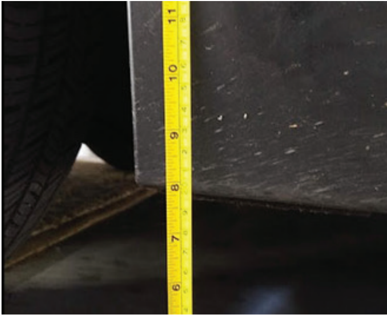
Front Suspension : Ground clearance before installation 7"
