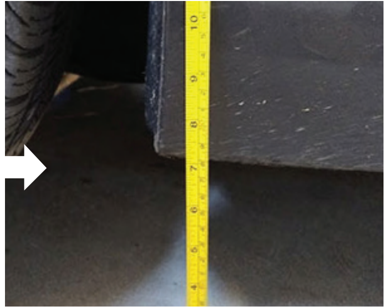
Front Suspension : Ground clearance before installation 7.9"
