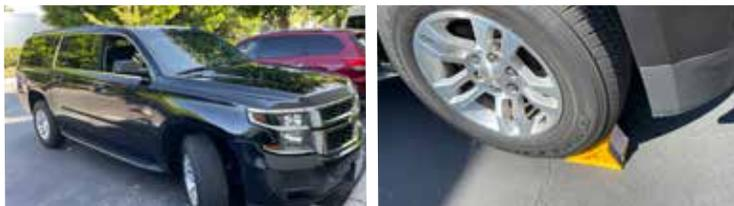
Note : Always put a wheel stop on the front end before installation.
