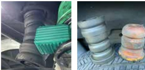
3. Add MUB2 x2 to provide extreme support for under heavy loads and increase ground clearance. Approximately 1", From 38"->39".
