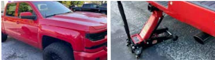
**Tip** : Jack up the truck for easier access to remove and install the bump stops.
