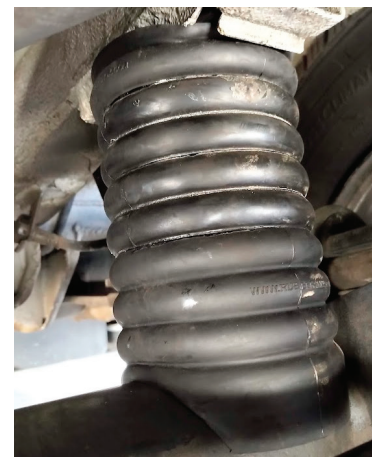
RubberShox UB1A223A Installed under 2015 Mercedes Benz Sprinter 2500 (2016 RoadTrek SS Agile) Rear Suspension
