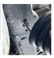
Pick the shortest screw for F150 installation
