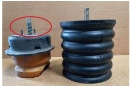
Original F150 factory bump stop VS RubberShox heavy duty natural rubber bump stop UB13
