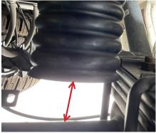
UB13 will be the best choose for occasional loading and towing with F150 truck. Our UBS series bump stops are direct fit with all Ford F150 truck without needing any alternation or adapter. For constant loading or towing, please choose UB123 for best stability and support of the vehicle without damage your truck (frame hitting the axel).
