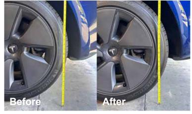
Ground clearance before installation -23.5" to reference line. After installed the UCSBM1,2, and 3 assembly, the ground clearance increased 0.5".
