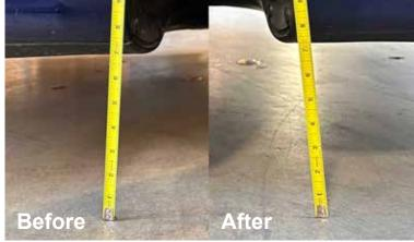
Before installing the from buffer, the ground clearance is 7". Ground clearance after installed UCSBH1 and UCSBH4 – 0.5" increased
