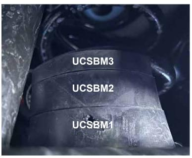
We installed UCSBM12344 for rear coil springs. UCSBM1, 2 and 3 modules are assembled to install in the rear coil springs.
