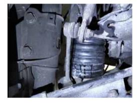
4. Use Pliers to guide SS stud and rotate UB122 to insert the included 45mm full threaded SS stud into UB122 (insert depth ~ 1.2")
