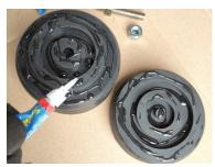
1. Glue and Combined models UB1+UB2+UB2 together (make sure hard heavy compress to join all item interlock completely with Glue preapply)
