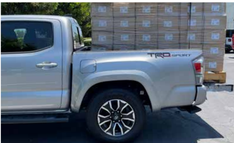
After loading 1,180 Lbs. weight. The truck slant to end rear.
