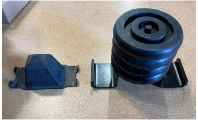
Difference between RubberShox UBS Bump Stop with factory original equipment.
