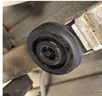
UB1A Replace to OE Bump Stop 2015 Mercedes Benz Sprinter 2500 (RoadTrek SS Agile) Rear Suspension (Require UB2 & UB3A Module)
