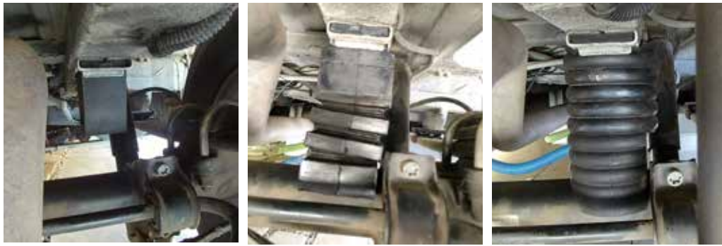
Showing OE Bump Stop vs. Other Brand vs. UB1A223A (2015 MB Sprinter 2500 / 2016 RoadTrek SS Agile)
